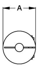
A = 122 D1 = 50 D2 = 50 L = 123 Nom. torque NM (Tkn) = 500
